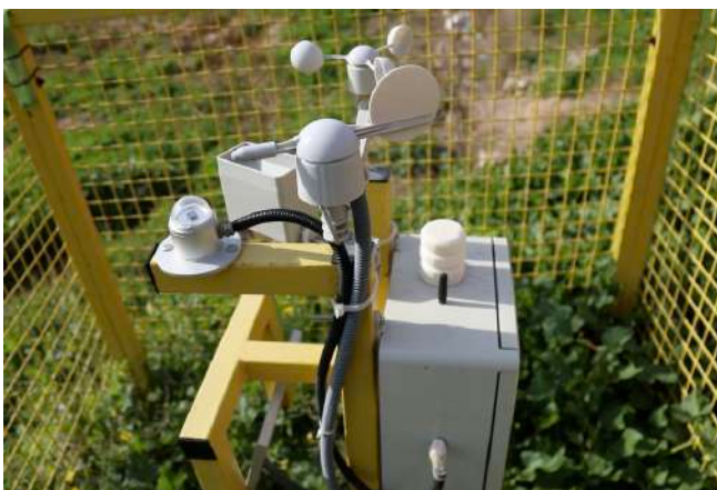
Figure 4 – Connected agro-meteorological station with integrated simulator for real-time monitoring of the weather parameters and automated calculation of the crops' water requirements.
